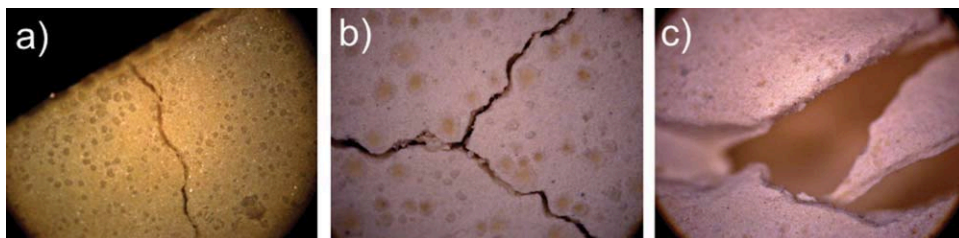
Figure 6. Kaolin samples dried with different MwP levels: (a) 120 W, (b) 180 W and 240 W, and (c) 300 W.
